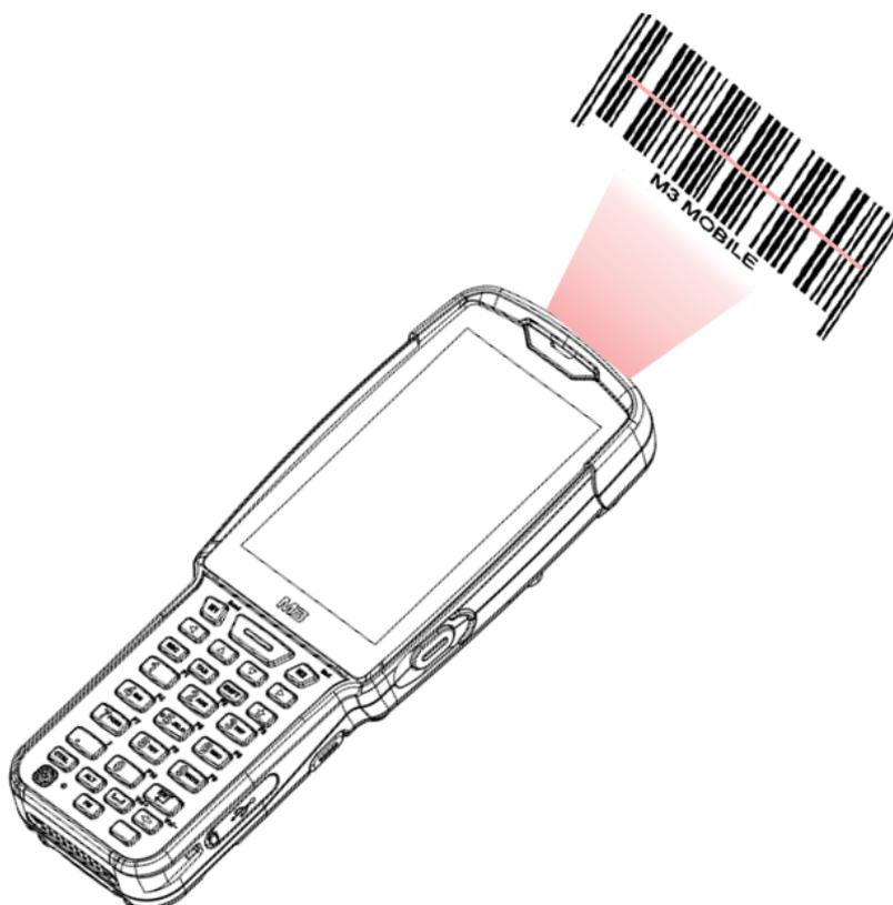
The laser beam of the scanner should completely cover barcode as shown in the following.
