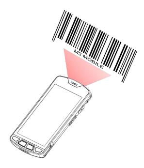
The laser beam of the scanner should completely cover barcode as shown in the following.
