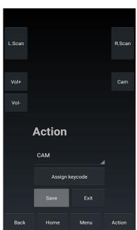
The setting of the device's physical buttons, except for Power button, can be changed.
