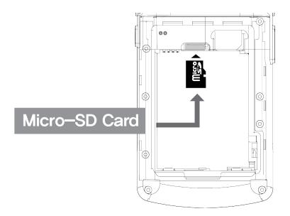
To insert Micro-SD card, Remove battery cover on the rear of the device and pull out the battery.
